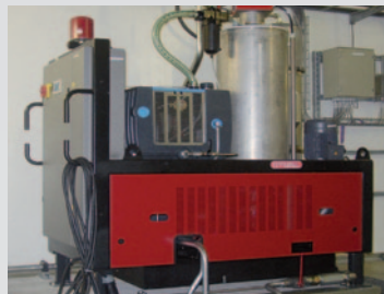
FAM FluidAquaMobil mobile unit for dewatering, degassing and filtration
