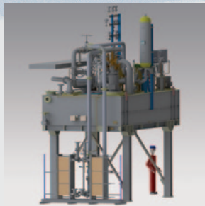
Bearing lubrication and lift system
