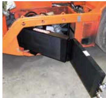
Combination cooler for drive motor cooling
