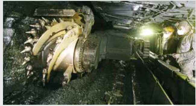
Longwall extraction with shearers
