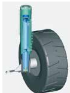
Cylinder for the loader suspension system
