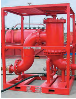
Oil and gas pipeline flooding with fresh water or seawater. Backwashing Filters AutoFit® RF3 are used to protect the flooding pumps
