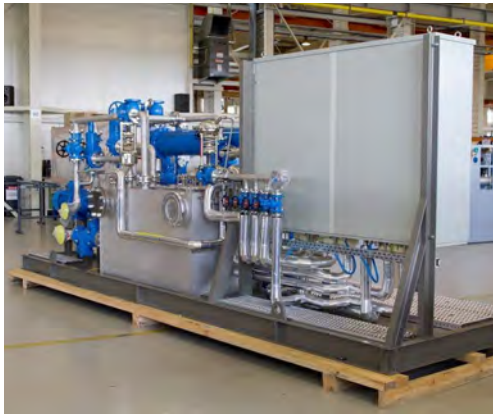
Lube Oil Systems as per API 610 & 614
