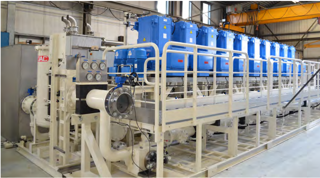
This HPU drives a hydraulic pile hammer for placing foundation piles subsea, for instance for offshore platforms or windmill foundations.
