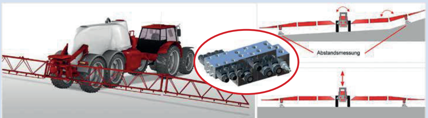
01 Ultrasonic distance sensors and highly dynamic valve and control technology provide slope and distance control for a spraying rod system
